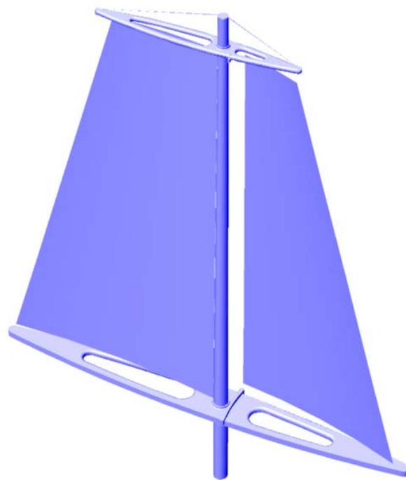
Fig. 3. Balanced rig example (source: [37])
