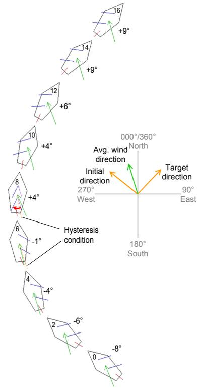
Fig. 6: Jibe from test run in 2 s time interval: rudder and sail position, apparent wind direction, heeling in deg, time from beginning in s.
