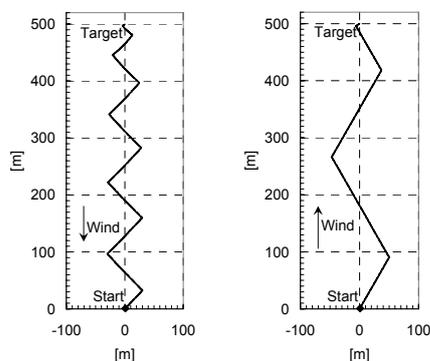
Fig. 4: Tack (left) and jibe (right) examples on a 500 m upwind/downwind course based on routeing method proposed by Stelzer and Pröll (2007).
