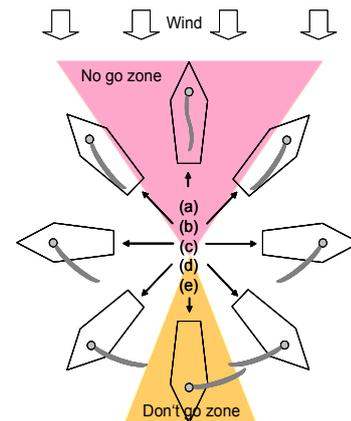
Fig. 2: Points of Sail: (a) In Irons (into the wind), (b) Close Hauled, (c) Beam Reach, (d) Broad Reach, (e) Running Downwind.
