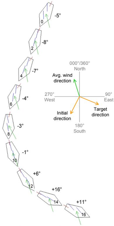
Fig. 5: Tack from test run in 2 s time interval: rudder and sail position, apparent wind direction, heeling in deg, time from beginning in s.
