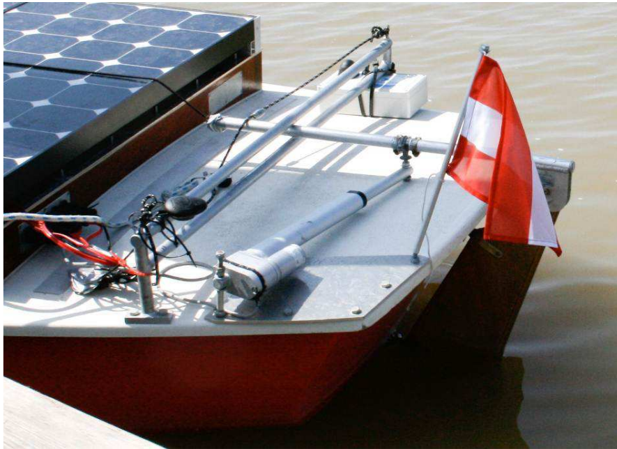
Figure 6 Linear actuator connected to the tiller controls rudder (2006–2008)
