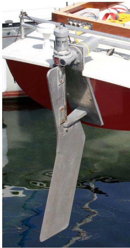
Figure 7 Self-constructed rudder gear with balanced rudder (since 2008)
