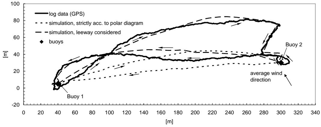
Fig. 15. Actual Run and Comparison to Simulation Results Based on Real Wind Data
