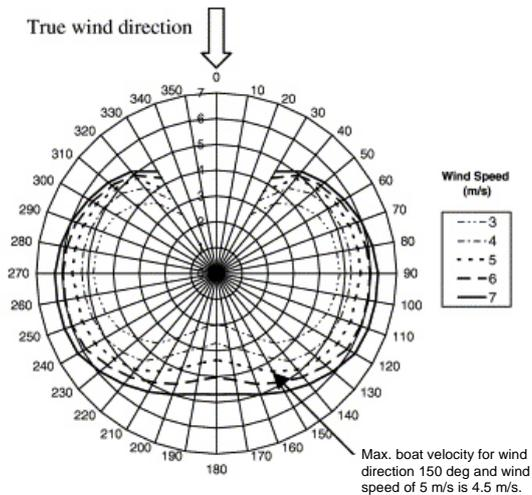
Fig. 1. Example of a Polar Diagram [11]
