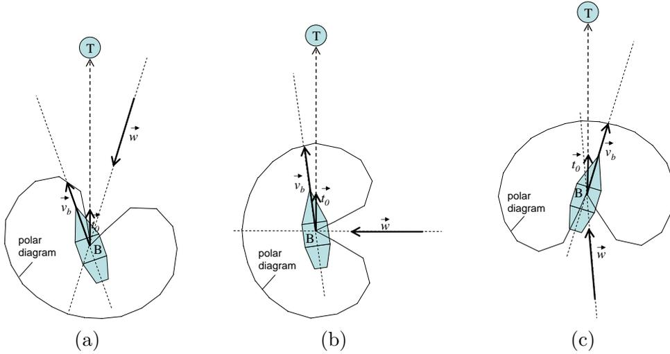
Fig. 2. Possible Constellations and Definition of Velocity Made Good
