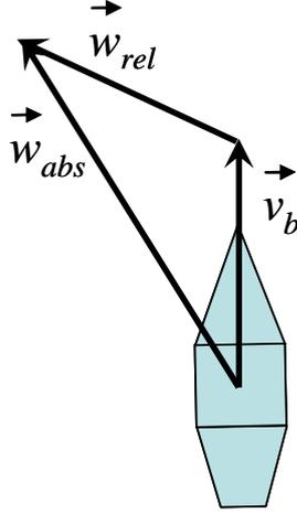
Fig. 9. True and Apparent Wind
