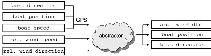
Fig. 8. Sensor Data Processing
