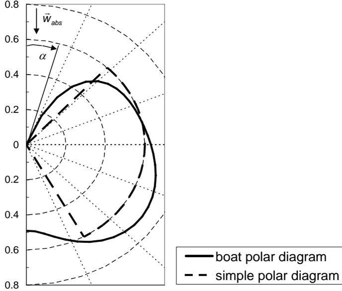
Fig. 10. Normalised Polar Diagram Used Within the Present Work (According to Eq. (9) and Table 1 for Unit Wind Speed)
